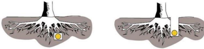
Figure 1: Tunnel to minimize root damage (left) as opposed to surface-dug trenches root zone (right)
