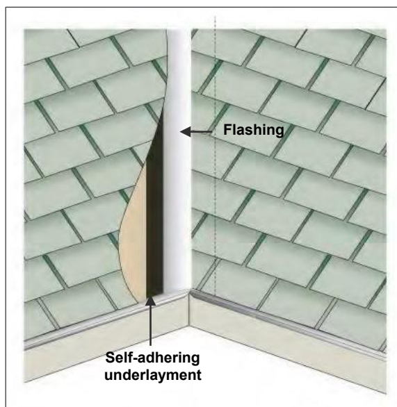
Flashing at Roof Valley
